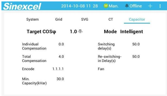
Figure A- 62 Capacitor settings information
