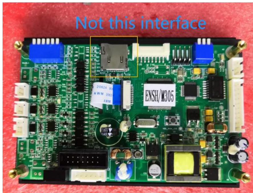
Figure A- 31 The position of SD Card Insert Interface
