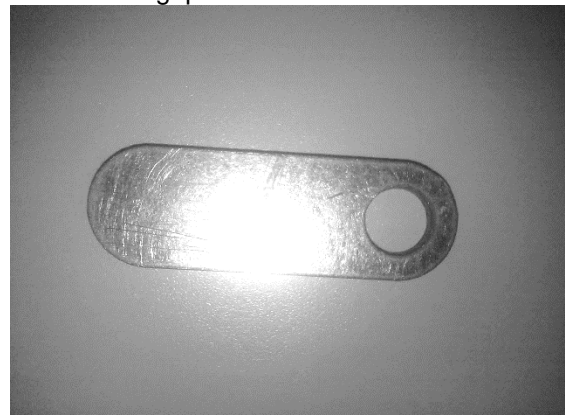
Figure 9: Gap tool (PN 43T02814-0020)
